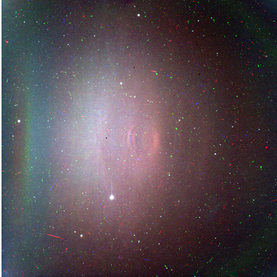
Figure 13: Contrast-enhanced color image of out-of-field stray light with the Sun as a light source. The (R, G, B) color channels represent filters (F5, F6, F3). Images were not divided by a flat field. The numerous colored specks and streaks are cosmic rays; only white objects are stars.
